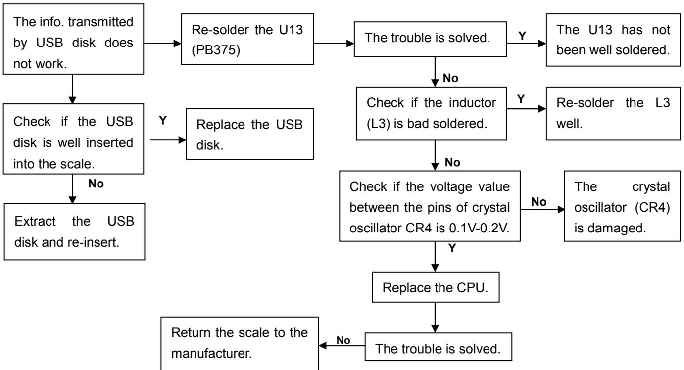
**Note:** Sometimes the scale is affected by its operating condition such as the climate or temperature; it may show error messages during the operating process.
