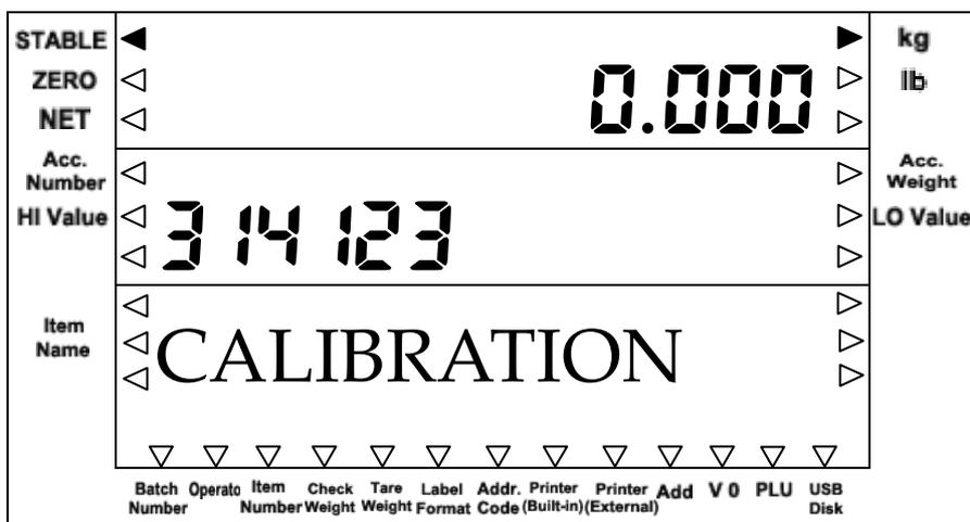
Press **Enter** key again to confirm the current “Zero Point”. The value will flicker for 3 seconds and then the weight for the first Span will be displayed.
