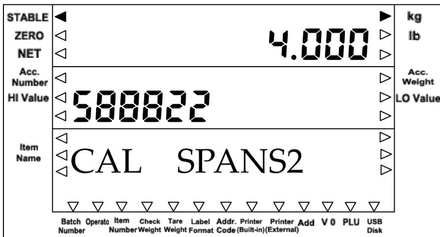
Put the weight exactly the same as the displayed weight value on the platform. Press **Enter** key once the display is stable to take sample for the current weight. The display will flicker and 2s later, the sampling procedure is finished. The third calibration weight will be displayed.
