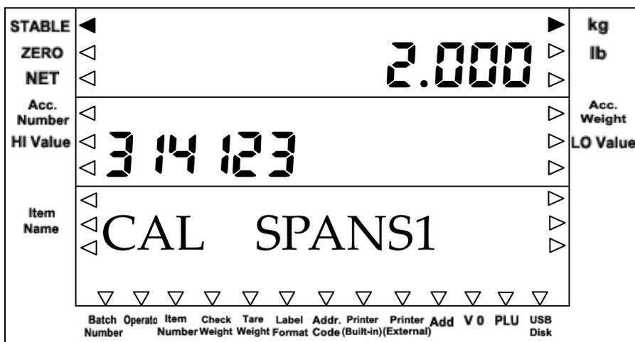
Put the weight exactly the same as the displayed weight value on the platform. Press **Enter** key once the display is stable to take sample for the current weight. The display will flicker and 2s later, the sampling procedure is finished. The second calibration weight will be displayed.
