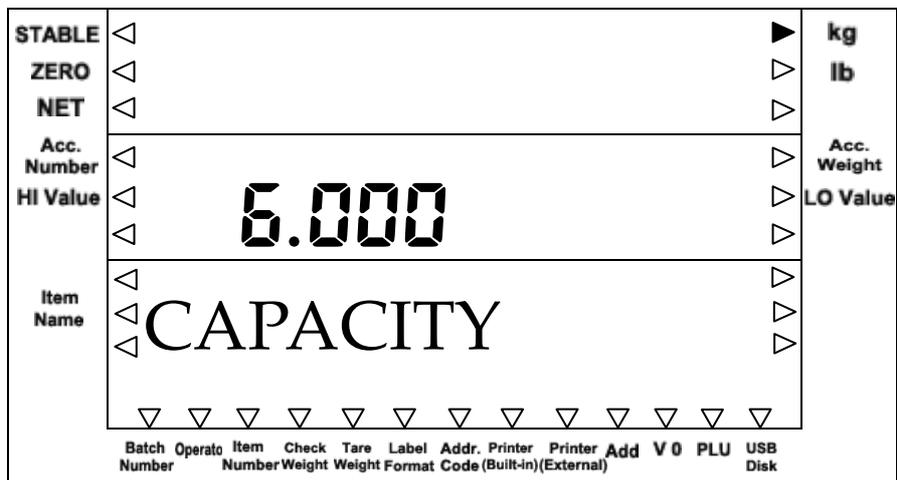
Press **Left** or **Right** key to move the “dot” position to select the capacity.
