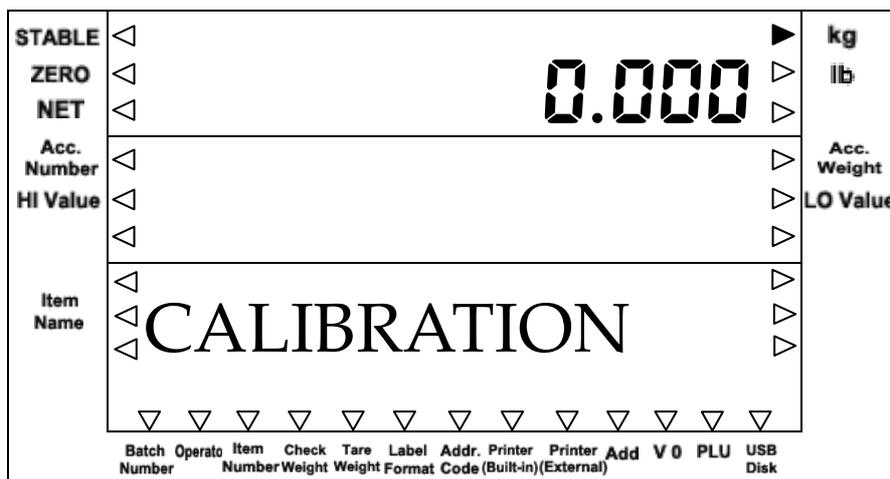
Give a long press of **Zero** key until the display shows as below:
