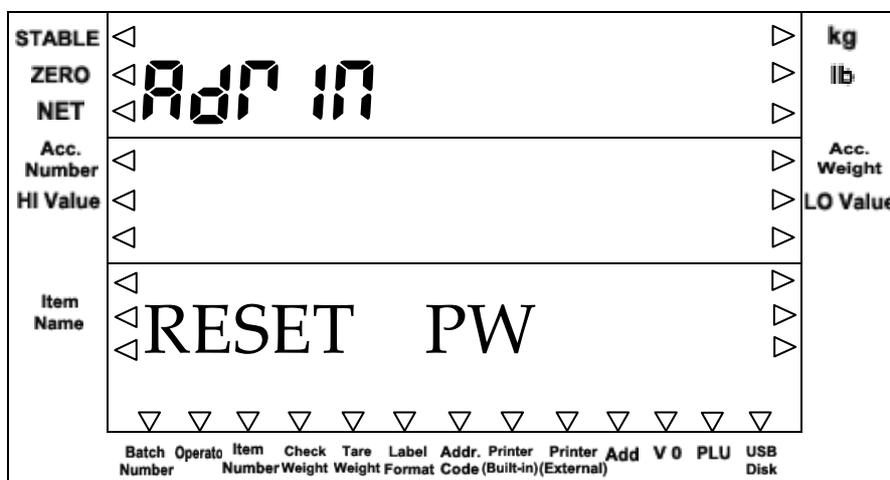
Press **Enter** key to reset the Factory Password "123456", then the display shows as below and indicates the reset operation is ok; press **ESC** key to return to last interface without reset the password.
